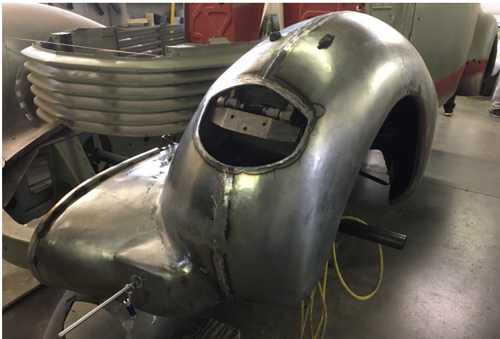
Fender of 1930's Cord showing extensive work
