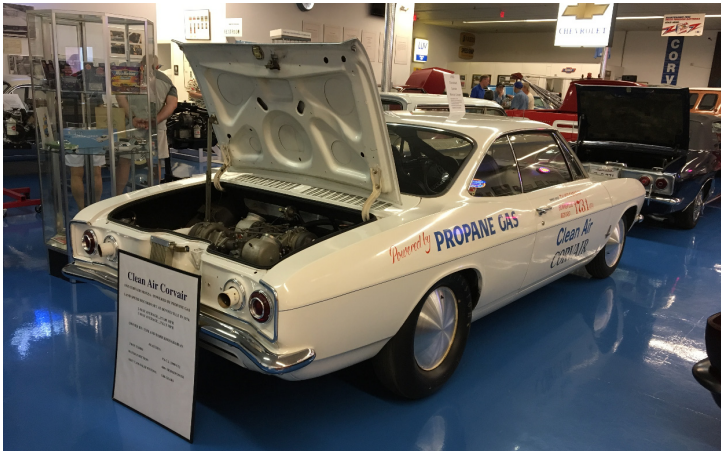
Clean Air Corvair is a 1965 Monza powered by propane. It has twin turbochargers with water injection. The 176 ci engine is rated at 400+ hp. With 3.08 gears it averaged 173 mph at the Bonneville Salt Flats in 1974.
