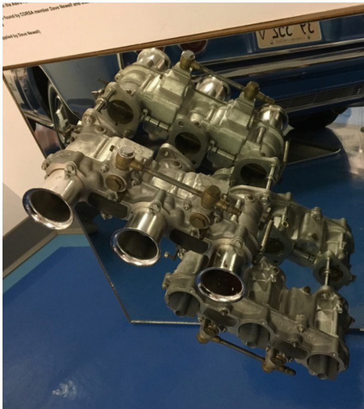
GM experimental 3 barrel carburetors pulled 170 hp at 5600 rpm. If GM had approved for production, it would have replaced the turbocharger already in production. They are mounted on a mirror sitting behind Corvair #5999.
