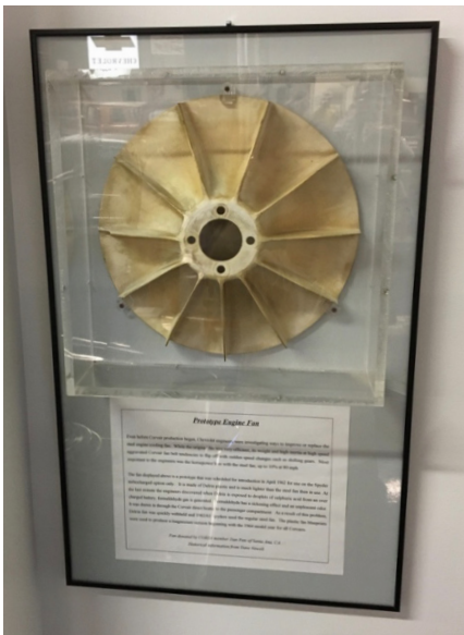
A prototype engine fan shown here is made of Delrin plastic, much lighter than the steel fan. GM engineers were studying ways to overcome the tendencies of fan belts flipping during sudden speed changes. They also discovered the Delrin plastic, when exposed to sulphuric acid from an over charged battery produces formaldehyde gas so a magnesium version was used beginning with the 1964 model year.
