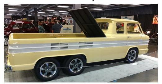
looks like a pretty neat vehicle. It is called a Corvadillac as it is powered by a 1996 Cadillac Northstar V8 engine with a four speed automatic transmission. The tag axle is also from the Cadillac.
