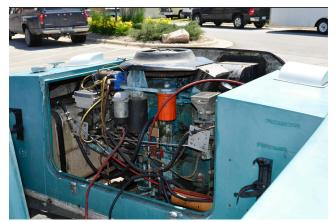
in the rear-engine Chevrolet Corvair of 1960. The engine has six cylinders arranged in a horizontally-opposed boxer configuration. The Turbo-Air 6 was used in the Corvair and all models derived from it, as well as a wide variety of other applications.
